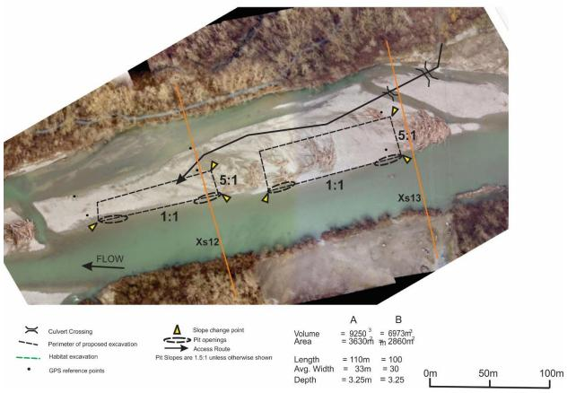
Figure 4: Yarrow Bar excavation.
