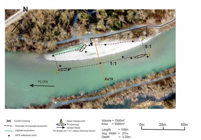
Figure 3: Railway Bar excavation.
