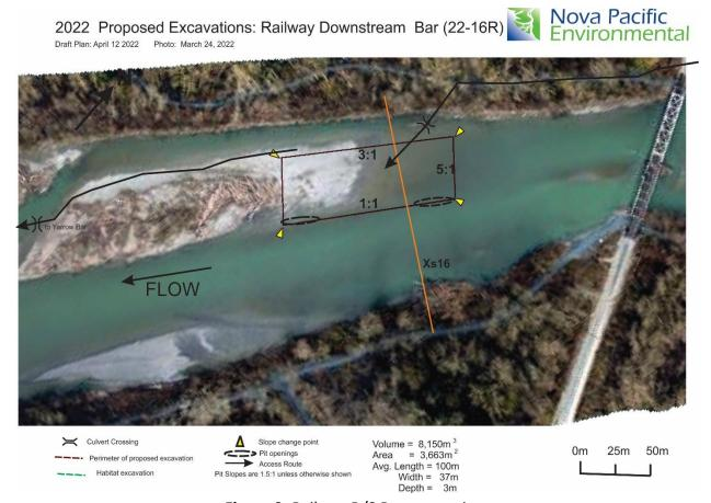
**Figure 9:** Railway D/S Bar excavation.
