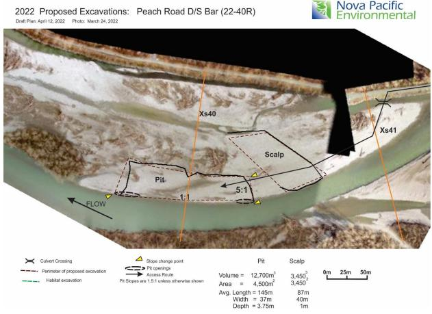
Figure 9: Peach Road D/S Bar excavation and scalp.
