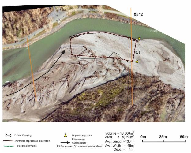
**Figure 2:** Giesbrecht Bar excavation.
