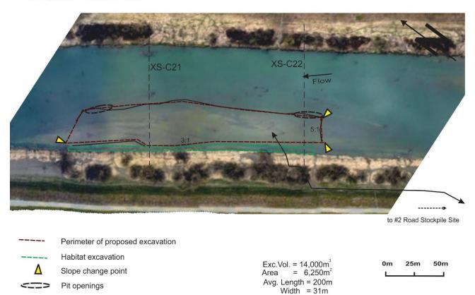
Figure 8: Boundary Bar excavation.
