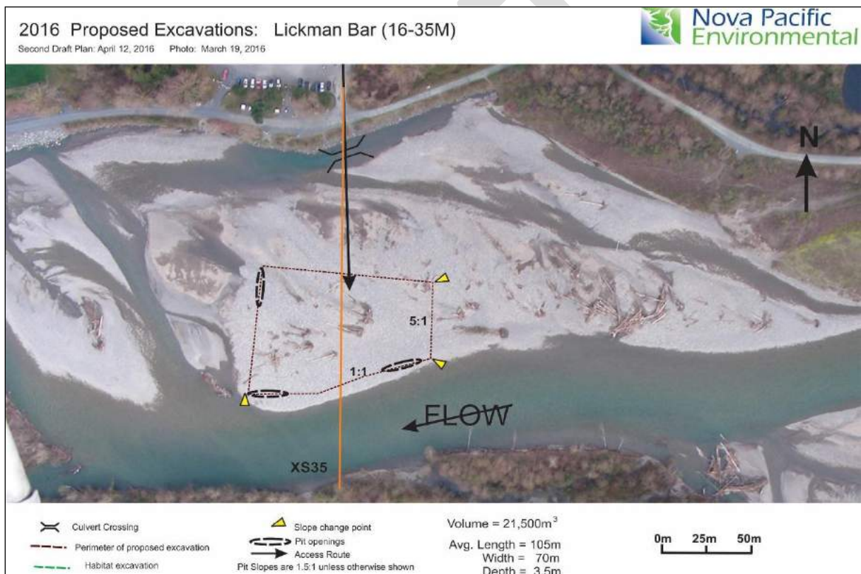
Figure L1: Layout of 2016 Lickman Bar (16-35M) sediment removal project. Photo taken March 19, 2016, draft plan – April 12, 2016.
