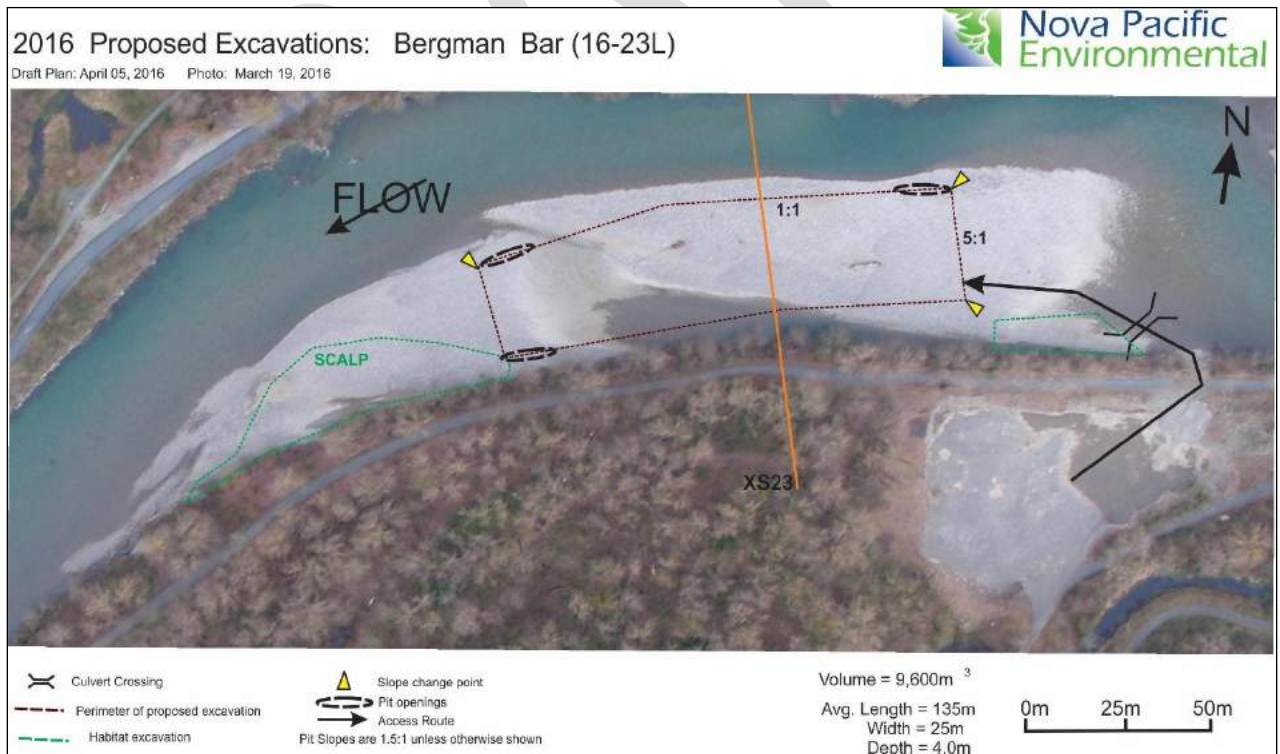
Figure B1: Layout of 2016 Bergman Bar (16-23L) sediment removal project. Photo taken March 19, 2016, draft plan – April 5, 2016.
